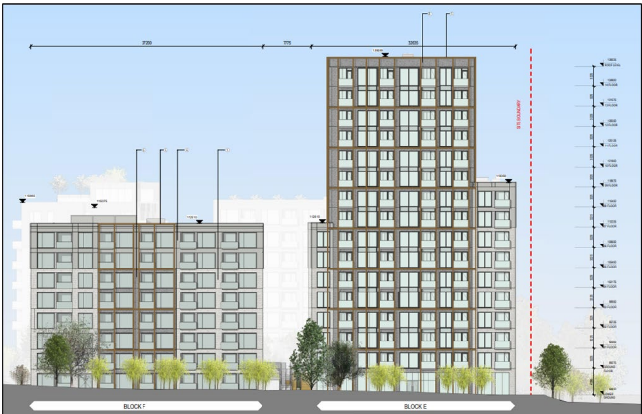
Figure 3: Building Height at tallest part of Proposed Development (North-East Elevation). MDO Architects
